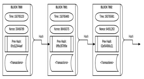
Figure 2: Mining a New Block to Insert into Blockchain
